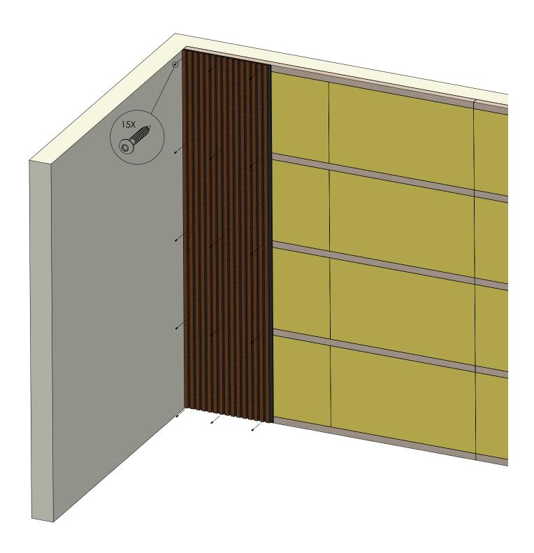
There are different ways to mount Ribbon. You can screw or glue the panels on existing walls / ceilings. If you want even better acoustics in the room, you can unbolt 45x45mm wooden rule and set insulation (45mm) in between, then you achieve sound class A.
