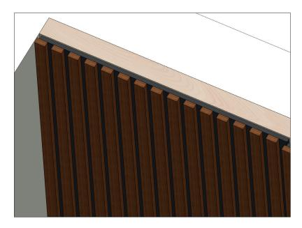
Screw up the panels on the wooden rule. 15 screw/panel.
