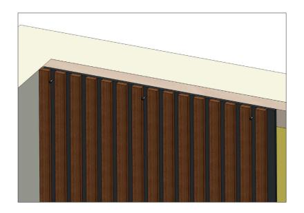
Screw or glue up the panels directly on the wall.
